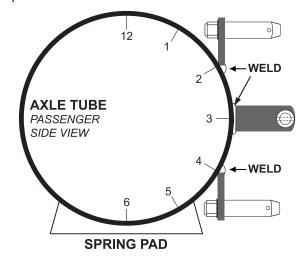
HINT: For easiest operation, the tapered mounting post should point forward as illustrated in the 2- or 4-o'clock configuration.
