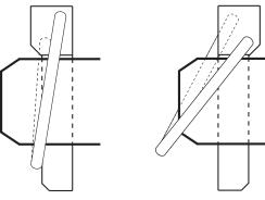
IMPORTANT: When properly installed, the ring on the Click Pin will "snap" against the shaft of pin. When installed backwards, the ring does <u>not</u> fit snugly against shaft.
