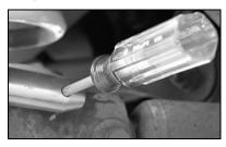
HINT: A small Philips head screwdriver or punch inserted into the Click Pin hole will enable you to prevent the Stainless Steel Post from rotating when tightening the mounting bolt.
