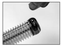
• Completely thread a Rod End (B) on to each end of Connecting Rod.
