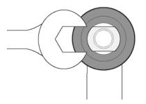
*HINT:* Use flat spot on Rod Ends (B) to prevent mounting stud from spinning when tightening 1/2" Flanged Locking Nut (D).
