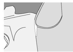
IMPORTANT: It should not be necessary to grind all the way through the steel bracket. Only remove enough material to eliminate the interference problem.
