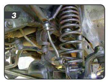
Disconnect the track bar from the frame rail bracket. Remove the cotter pin and nut (21mm) and thread it back on a few turns. Strike the track bar frame mount with a hammer to release the tapered seat. Remove the track bar.
