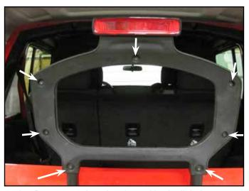
Remove and unplug the 3rd brake light by removing the two T25 screws.
