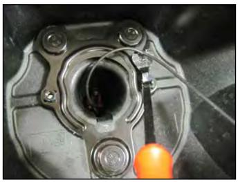
O Using a body clip tool or other appropriate tools pry the camera brack off of the spare tire mount.
