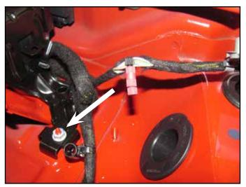
O Locate the provided wire. Strip both strands of wire on one end. Attach the red wire strand to the other end of the posi tap. Also crimp the ring terminal to the black wire strand. Place the ring terminal onto the seat belt bracket stud and tighten down the OE flange nut
