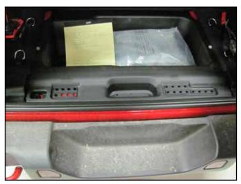
O Remove the passenger side tie down panel. Pry up the tab with a body clip tool. Then remove the bolt using a T40 bit on all 3 tie downs.
