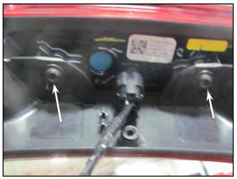
Remove the eight bolts holding on the spare tire mount.
