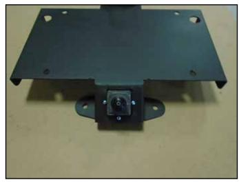
O Using the provided #8-32 machine screw and nut mount the new license plate light onto the top of the lincese plate bracket. Phillips screwdriver and 11/16 socket/wrench. Torque to 18 in-lbs
