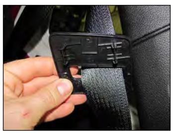
• Remove the rear corner body panel using a body clip tool. There are a total of 15 clips holding it on.
