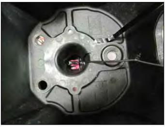
Once the camera mount is removed remove the 3 camaera screws T8 and disonnect the camera.
