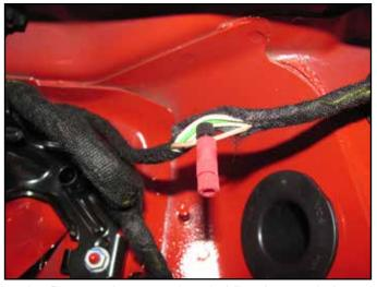
O Remove the serated nut holding the seat belt bracket to the tub. 10mm socket/wrench.
