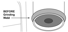
Carefully grind the circumference of the weld to match the major diameter of the upper spring retainer. Remove only as much material as is necessary to avoid disturbing the weld integrity.
