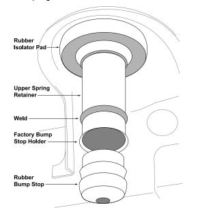
• Locate the factory weld that secures the bump stop holder to the upper coil spring retainer.
