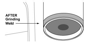
Remove any sharp edges from the cut portion of the upper spring retainer.
