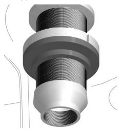
• Install Bump Stop Adapter (E) onto Threaded Tube (A) and tighten by hand until snug.
