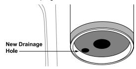
• Drill a 1/4" drainage hole in the bottom of the upper spring retainer as illustrated above.
