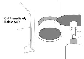
• Cut away the lower portion of the bump stop holder <u>immediately below</u> the weld. The weld itself must remain intact – use caution to avoid damaging it.
