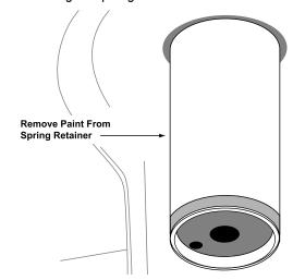
Remove all of the factory paint from the surface of the upper spring retainer.
