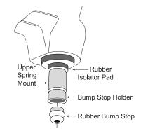
• Cut away the lower portion of bump stop holder until even with bottom of flat washer. DO NOT CUT OFF FLAT WASHER! *HINT*: A die grinder with cut-off wheel or reciprocating saw is useful for cutting bump stop holder.
