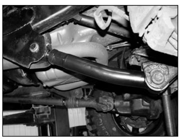
O Install the original mounting bolt and finger tighten the nut. Remember to realign cam adjuster on front axle if equipped. DO NOT torque mounting hardware until instructed.
