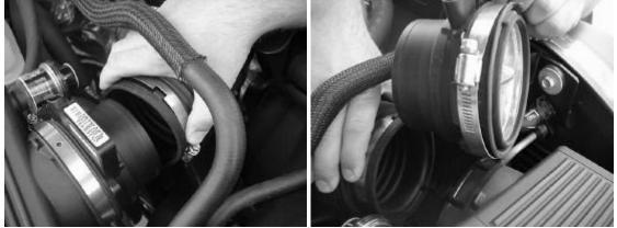
3.Remove gasket from stock Mass Air Sensor and install on Powr-Flo Sensor
