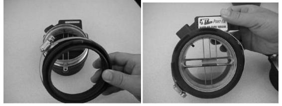
4.Install JET Powr-Flo Sensor, tighten all clamps and plug in harness Note: Some applications come with a adapter harness, this will plug into your factory harness. Only use if your application originally had a three wire harness.
