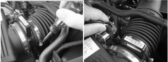
2. <u>Remove Intake Hose and remove stock Mass Air Sensor</u>
