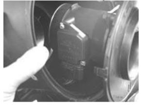
3. Remove stock Mass Air Sensor and Install Powr-Flo Sensor
