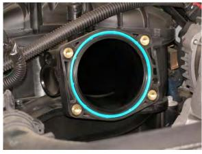
6. Use a 4mm socket to remove the top 2 studs from the intake manifold. The manifold should now look like the photo.
