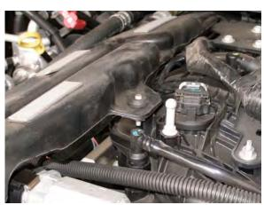
10. Reinstall intake tube over grommet being careful that it properly seats.
