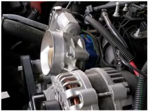
7. Install 4 supplied bolts and washers through throttle body, then gasket, then spacer and into manifold. Finger tighten at first, then use 10 mm socket to tighten.
