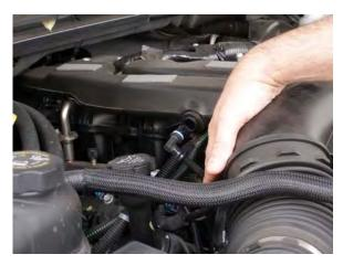
4. Disconnect breather tube from intake by gently pulling outwards. Loosen clamp at mass air sensor then remove intake tube.
