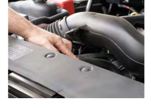
2. Loosen the clamp securing air intake tube to the throttle body.
