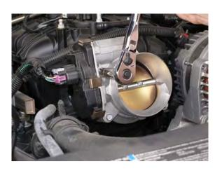
5. Use a 10mm socket to remove the 2 nuts and 2 bolts securing throttle body to intake manifold. Set throttle body aside without disconnecting the wires.
