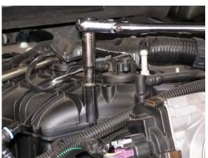
8. Remove ball stud that secured intake tube to manifold. Install allen bolt in countersunk hole in extension plate, then install on manifold and point towards front of motor. Install factory ball stud in hole on other end of extension plate. Tighten countersunk bolt and ball stud.
