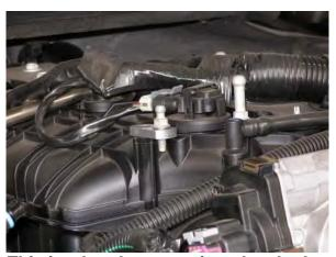
9. This is what the extension plate looks like installed. Remove the grommet that installs over ball stud from intake and install it on ball stud with the small diameter size facing up. This will make installing the intake tube much easier.
