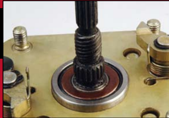
Caged Needle Bearing Supported Drive Pinion
