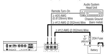
Route all power wires through grommets in the vehicle's firewall. If factory grommets are not available, install grommets yourself. Connect a short ground wire from the GT-BassPro12's ground terminal to the nearest bare metal surface on the vehicle. For a good connection, use sandpaper to clear the paint from the metal surface and use a screw with a lock (star) washer.
