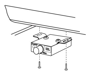
Route the supplied remote level control cable behind the dashboard or other interior panels and under the carpet. Do not route the cable outside the vehicle. Connect the cable between the GT-BassPro12's Remote Level Control connector and the connector on the remote level control.
