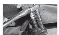
6. Remove oxygen sensor using a 12mm socket, save gasket.
