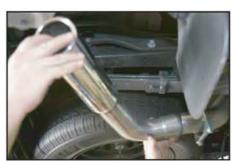
12. Install turnout onto axle pipe
