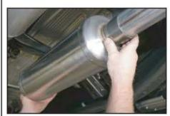
9. Install muffler onto axle pipe
