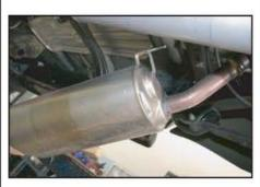
7. Remove muffler assembly from vehicle
