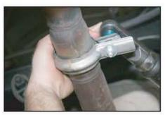
4. Remove clamp behind muffler
