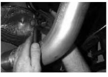
11. Insert the tail pipe hanger into the rubber grommet behind the muffler.
