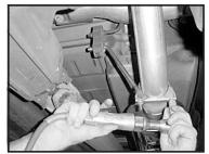
9. Install muffler hanger clamp (D) at the rear of the muffler. Align tailpipe (B) properly and secure.
