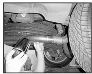
10. Slip tip (C) onto tail pipe (B).
