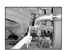
11. Align the tip properly and tighten clamp.
