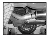
7. Insert tail pipe (B) into muffler (A).
