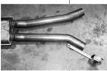
3. Using pliers or a pry bar, slide the rubber hangers from the hanger rod on the muffler and tailpie (a little WD40 helps). Remove the muflers from the car
