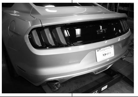
JBA recommends taking the vehicle to a muffler shop and having all slip connections tack welded.
