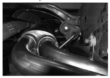
15. Manipulate the tailpipes and mufflers so that they are level from the passenger side of the truck. When you are satisfied with the position tighten all the clamps, making sure that the tips stay aligned as you do.
