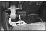
4. Spray lube on rear tail pipe hanger rod and remove from lower hole in rubber grommet using channel lock pliers.
