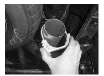
17. Install exhaust clamp (H) loosely over tail pipe (C). Do not tighten at this point.
