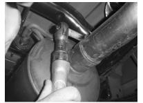
3. With the vehicle raised and properly supported, using the 15mm socket and ratchet, loosen the clamp, at the rear of the muffler, that secures the tail pipe to the muffler.
