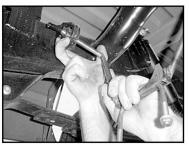
9. Install the muffler hanger clamp (E) in to the factory rubber isolators with hooks facing rearward. Slip outlet of muffler (B) in to hanger clamp (E).
