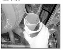
13. Slip 3" clamp (F) over the rear of axle pipe (C).
