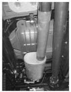
10. Install the JBA muffler (B) with the off-set inlet toward the center of the vehicle on to intermediate pipe (A).
