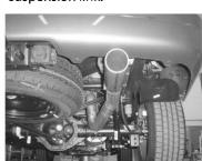
16. Align the tail pipe with tip (D) as shown for proper clearance on the rear bumper.
