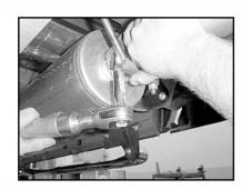
17. With the tail pipe (C) and axle pipe (D) aligned properly, tighten muffler hanger clamp (E) and rear clamp (F).
