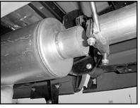
13. Slip axle pipe (C) through muffler hanger clamp (E) and in to outlet of muffler (B).
