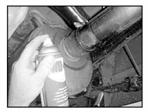
4. Spray lubricant on the exhaust pipe behind the muffler.
