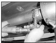
11. Place 3" exhaust clamp (F) at the front of the muffler and securely tighten.
