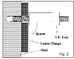
13. As with the driver's side, apply anti-seize to the bolts, apply silicone to the dome flange, and bolt the headers to the head and the exhaust system. Reattach the spark plug looms in the same manner as the driver's side.
