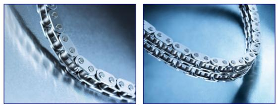
Simplex and duplex roller chains with a 3/8" pitch are used primarily in timing drives, oil pump drives and drives for auxiliary units, especially for petrol engines. Owing to its smaller pitch, a roller chain with an 8 mm pitch cuts the weight and consequently reduces the centrifugal forces and impact speed. It is therefore ideal for downsizing to timing drives with moderate loads.
