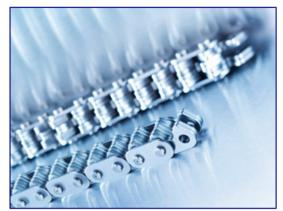
The meshing of the toothed links with the sprocket gives this chain optimum acoustic properties for timing drives where acoustics are crucial, especially for petrol engines. The 8 mm pitch is also suitable for higher load chain drives, while the low weight of the 6.35 mm pitch makes it ideal for downsizing timing drives with moderate loads.
