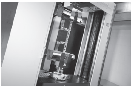
Evaluation of chain breaking strength and elongation up to 1000 kN
