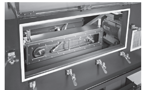
Testing of chain wear elongation behaviour on more than 20 test rigs
