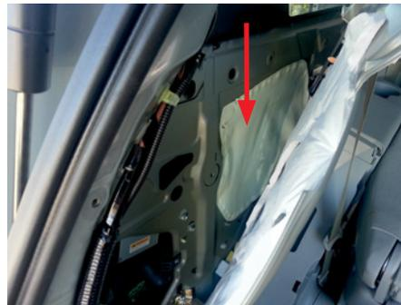
Pull back the plastic and access the satellite tuner plug
