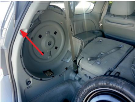
The satellite tuner connector is behind the plastic
