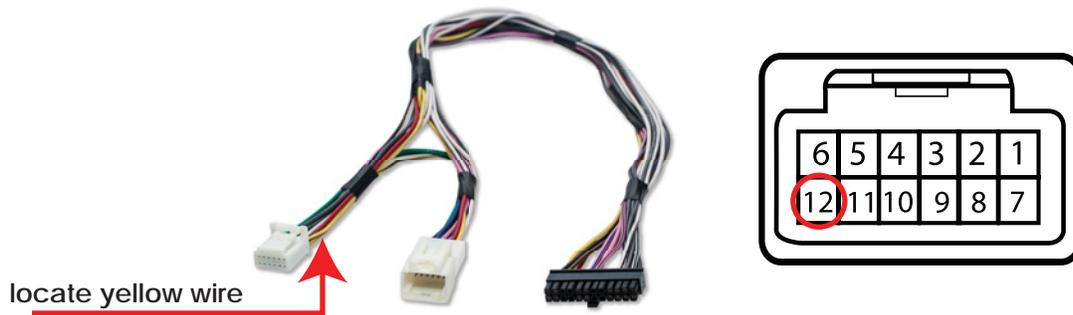
Depending on the vehicle, the radio will have one of the two types of harnesses at the radio to use for the battery 12 volt connection.
