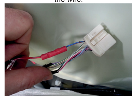
Make the connection as shown here using the supplied crimp connector. Insulate and secure the other side of the wire.
