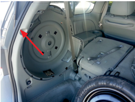
It should now look like this. Pull on the panel from the back edge to release it.
