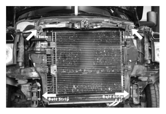
D) Remove four 18mm nuts and two bolt strips holding OEM bumper to frame rails. Diesel only: Move one side of intercooler at a time to remove bolt strips (Picture #2). NOTE: Be careful not to damage intercooler fins.
