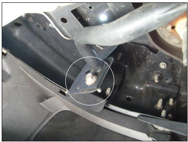
2. Remove nuts from factory U bolt.
