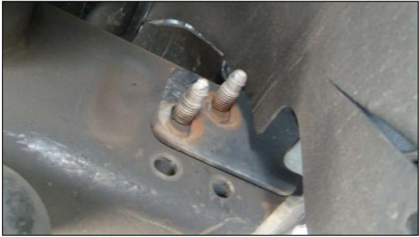
3. Remove hardware connecting tow hooks.
