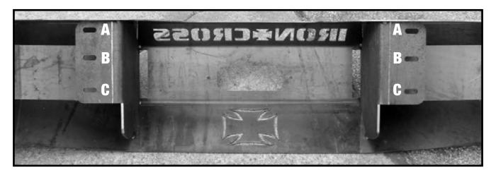
A. ALIGN BUMPER MOUNTING HOLES (A,B,C) TO BUMPER BRACKET HOLES (A,B,C). B. INSTALL HARDWARE AS SHOWN. HAND TIGHTEN HARDWARE AND LEAVE LOOSE TO MAKE ANY ADJUSTMENTS.
