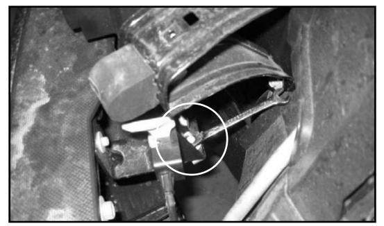
D. REMOVE FRONT BUMPER REAR BRACE BOLTS
