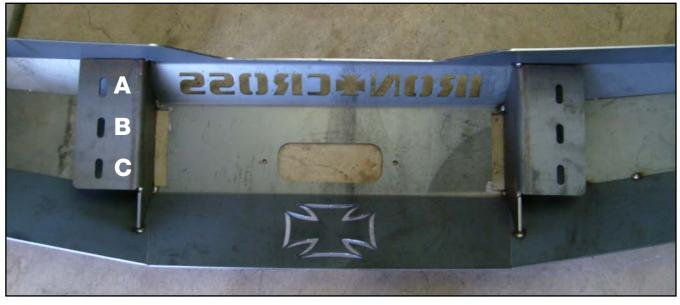
ALIGN THE BUMPER SIDE TO SIDE AND TOP TO BOTTOM TO ENSURE A PERFECT FIT TO THE TRUCK. ALLOW FOR A 0.25" CLEARANCE TO ALL PAINTED SURFACES IF POSSIBLE TO ALLOW FOR FRAME FLEX.
