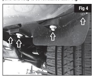
**4.** Remove the (3) screws attaching the inner fender panel in front of the front wheel. Keep for reinstallation. **Fig 3**
