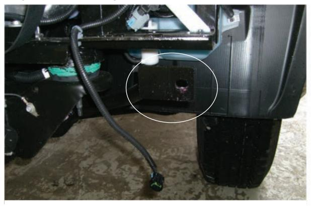
C. Remove 21mm nuts(2 Per Side) FASTENING TOW HOOK, 1 on bottom and U-BOLT from the frame holding the bumper brackets to the frame. SUPPORT BUMPER BEFORE REMOVING BOLTS.
