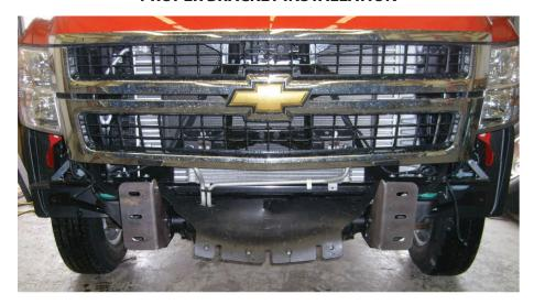
On some models, you may need to remove the rubber trim from the top of the bumper that goes underneath the headlights. Trim rubber to length to fit the Iron Cross bumper properly.
