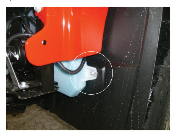
E. Pull outward slightly at the fender wells and remove the bumper from the front.
