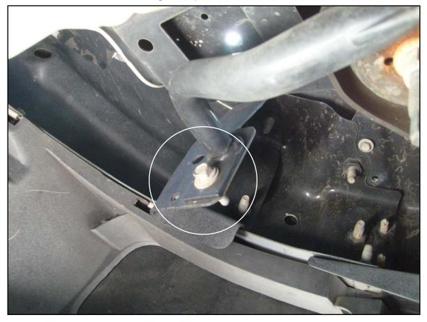
2. Remove nuts from factory U bolt.
