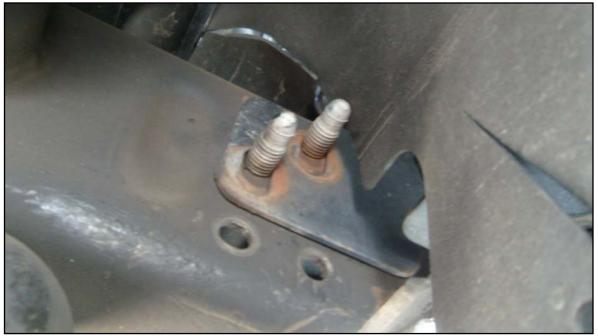
3. Remove hardware connecting tow hooks.
