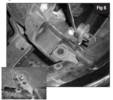
I) Remove (2) bolts from each side of frame holding bumper to frame. Be sure to place oor jacks or have a person hold bumper once these bolts have been removed. Fig 7.
