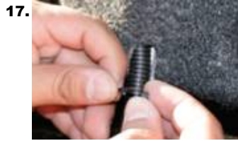
Zip tie (Gray) wires to stock wire harness.
