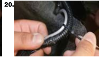
Zip tie (Gray) wires to stock wire harness & reinstall (IPCW) taillights.
