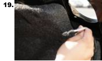
Then connect wire to the trunk lid light.
