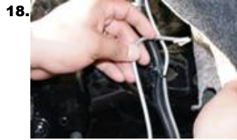
Run passenger side (Gray) wires thru the inner panel of the trunk lid.
