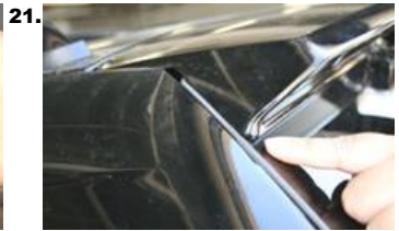
21. Recheck upper moulding ass'y and liftgate alignment..
