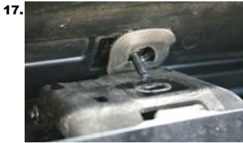
17. Install moulding ass'y on liftgate. Make sure studs are through the hole on hinges.
