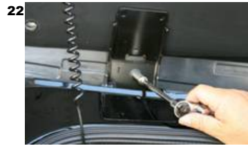
22. Tighten 2 ea. 10 mm nuts on hinges.
