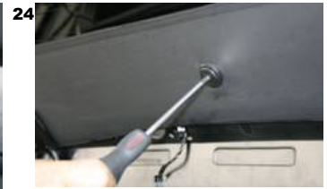
24. Install 3 ea. TORX head screw kept from step 3.
