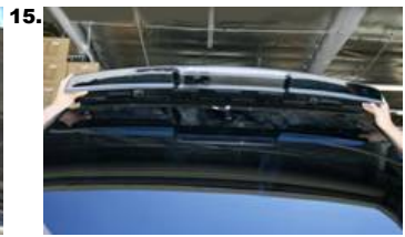
15. Put moulding ass'y to top of liftgate. Be careful not to damage paint and glass.
