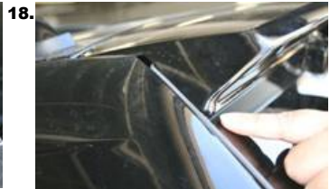
18. Check upper moulding ass'y to make sure it is aligned with liftgate.
