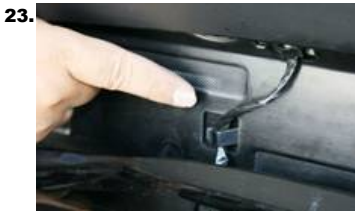
23. Tuck wire harness back behind clips.
