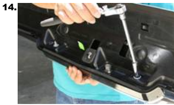
14. Install 2 each 10mm nuts kept from step 10 on IPCW 3rd Brake Light to moulding ass'y .
