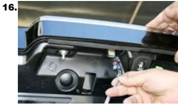
16. reconnect stock light plug to NEW LED 3rd brake light.
