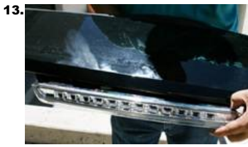
13. Install new IPCW LED 3rd Brake Light on moulding ass'y.
