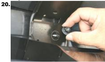
20. Install 2 ea. 10 mm nuts on hinges kept from step 5 . Hand tight only.
