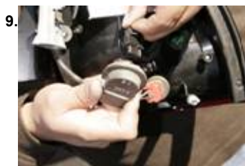
9. Plug in the bottom 3-wire male connector to vehicle's socket harness. Make sure to match black wire to black wire .
