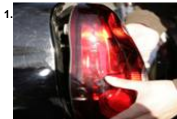
1. Open trunk and simply remove butterfly nuts using your hand and remove stock tail light.
