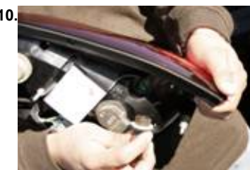
10. The small (194) socket would require no bulb, no wire connection, just twist & lock to seal the light.
