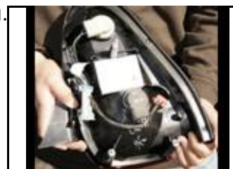
11. Before installing make sure everything is connected & tightly sealed.
