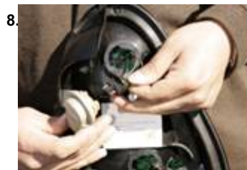
8. Plug in the top 2-wire male connector to vehicle's socket harness. Make sure to match black wire to black wire .
