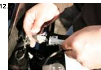
12. Now simply reconnect wire harness to vehicle factory plug and reinstall IPCW taillights on vehicle.
