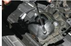
15. Remove all (3) screws on the back of stock turn signal.
