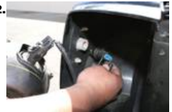
12. Disconnect the side marker.
