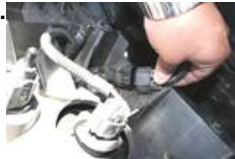
11. Disconnect from wire harness.
