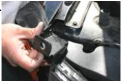
9. Remove the screw to release bracket.
