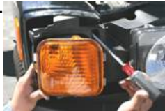
6. Unscrew the 10mm nut located in upper area of stock turn signal.
