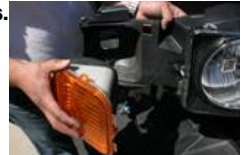
16. Remove stock turn signal.
