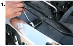
1. Unscrew (2) 10mm nuts above the grille on header panel.
