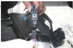
21. Connect L.E.D. light to stock socket. Make sure they match ( Black wire to Black Wire ).
