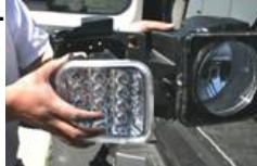
18. Place L.E.D. light onto the panel.
