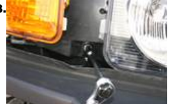
8. Unscrew the 10mm nut between headlight & lower area of stock turn signal.
