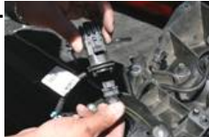
14. Twist & unlock socket and remove bulb.
