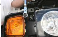
6. Unscrew the 10mm nut located in upper area of stock turn signal.
