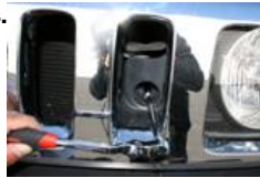
3. Remove the 10mm screws in the grille next to the headlights on each side.
