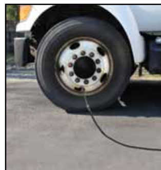
Inflate and equalize steer and drive tires simultaneously. #TEQ-5HLTC Lock-On Tire chucks are available separately.*
