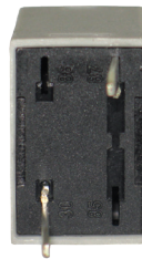
Small Spade Relay 2000 and Newer Domestic, Korean, and Japanese
