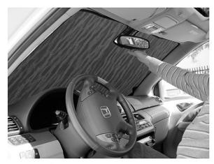
STEP 3: Lift the CUSTOM GOLD AUTO SHADE<sup>™</sup> against glass. Adjust the CUSTOM GOLD AUTO SHADE<sup>™</sup> in windshield, may overlap slightly with side windshield frame (A-pillars) and headliner.
