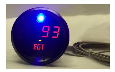
O The gauge can also act as a ground switch providing ground to an external device or relay that is required to be activated at your chosen temperature settings. This switch can be set as 'normally open' or 'normally closed' and has its own LED indicator.
