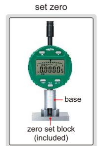
measure peak-to-valley height of blast cleaned surfaces
