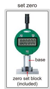
measure peak-to-valley height of blast cleaned surfaces
