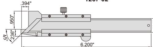
measure 45° chamfer dimension
