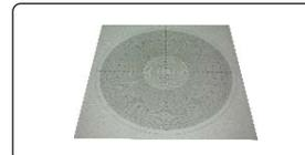
overlay chart (protractor with 1° graduation, radius with 1mm/.039" increment)
