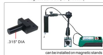
can be installed on magnetic stands
