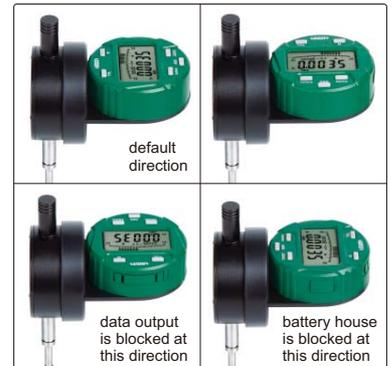
Remark: To change above direction, 4 fixing screws on the back of display need to be removed first.
