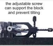
the adjustable screw can support the block and prevent tilting
