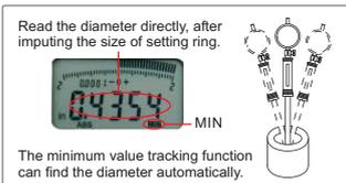
Read the diameter directly, after inputting the size of setting ring.
