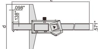
**MEASURE WIDTH AND DEPTH OF GROOVES INSIDE BORE**
