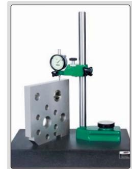
rigid construction, designed to make comparison height measurement (set zero with gage block then measure height of workpiece) with dial indicators or electronic indicators (variation of measuring force is high)
