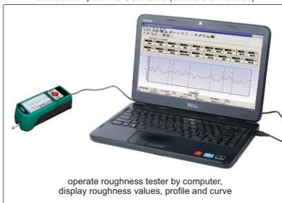
operate roughness tester by computer, display roughness values, profile and curve
