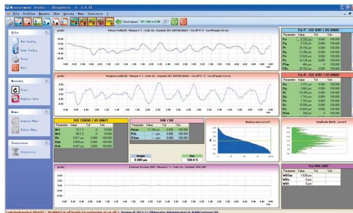
measuring software (optional), can control the roughness tester,
