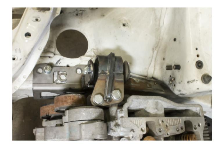
Finally, align and bolt up the rear mount with the rear mounting bracket. Keep the engine secured. You may need to torque or move the engine around until all mounts align with their corresponding bolt holes.
