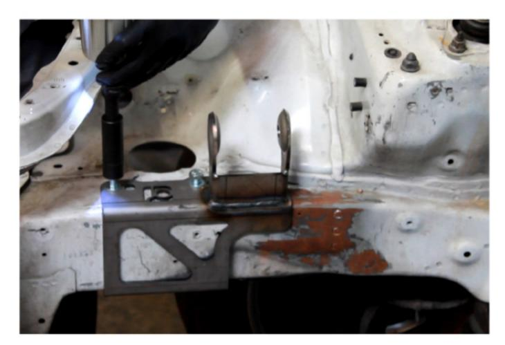
Bolt in the rear mounting bracket to the cross-member(90130-SB). Leave the bolts loose at this point
