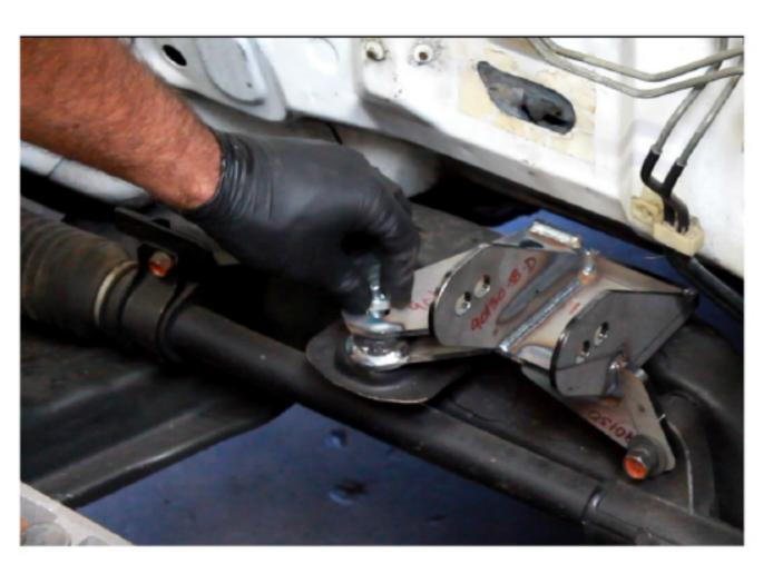
Place the transmission mount within the mount support on the driver side framerail, secure it with the OEM bolt.
