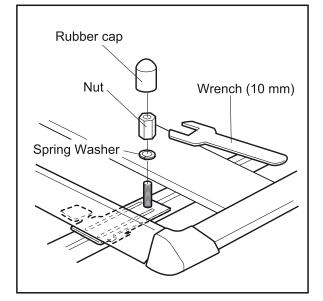
Using the installation part, nut plate and the hexagon socket head cap screw, tighten them. However, over tightening may result in deformation of the cargo basket.
