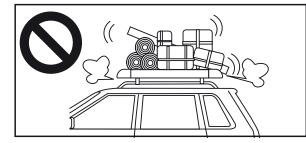
Do not exceed the maximum load capacity when loading. The maximum load capacity differs depending on the combination of the cargo basket and the vehicle model. Refer to the Fit Guide. Refer below for the method on calculating maximum load capacity.
