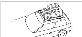
Be sure to securely fix the load with a belt, net, and/or rope. Travelling at high speeds or carrying a load weighing 22 lbs (10 kg) or more results in excessive force being applied to the load due to wind pressure and when starting or stopping the car. Always use a belt.
