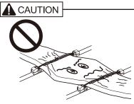
Tighten the ratchet securely, but avoid denting the board. Excessive tightening may cause damage to the board.
