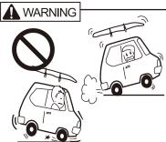
Do not make hard starts, unnecessary sharp turns, abrupt maneuvers or sudden stops. In case you have to perform such a maneuver, always check afterwards to see that the carrier and cargo remain secure.
