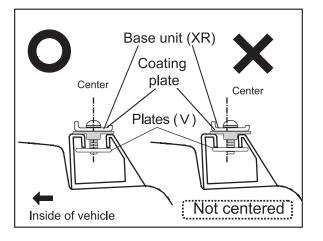
Tighten both bolts alternately using the attached Allen key.
