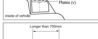
Be sure to keep the distance between the front and rear carriers more than 27.5inch (700mm).
