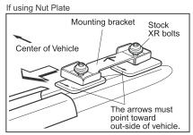
See Stay (IN-XR model) manual for assemble and mounting intrusion.
