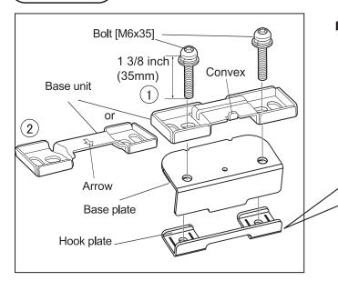
Attach the base unit, base plate and hook plate with 2 bolts[M6x35].
