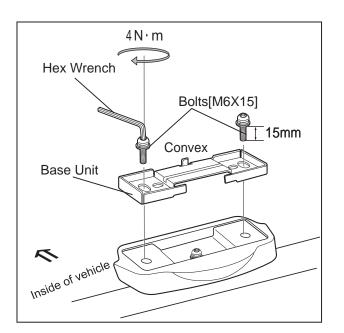
Place the base unit on the installed cushion base/base bracket. Then using the Hex wrench (included), tighten while alternating between the right and left bolts (short) [M6x15] (supplied with the carrier) until the bolts are firmly tightened.
